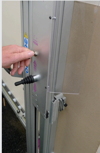
Push/pull button operates powerful pneumatic clamp
