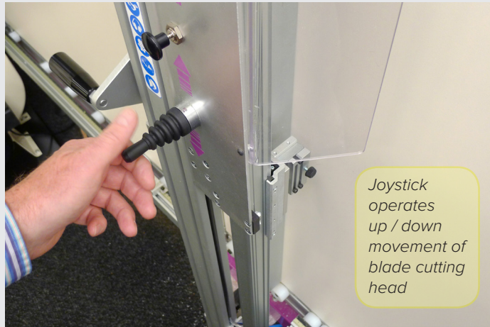
Blade cutting head powered by pneumatic linear actuator. Shown here with optional laser sighting system
