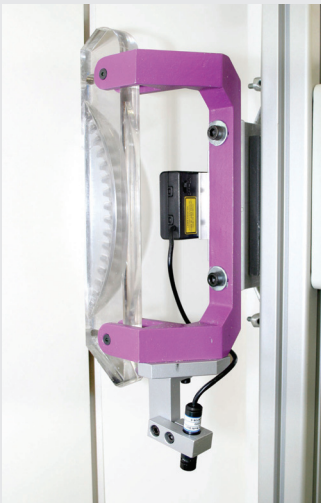
Saw handle, fitted with optional laser sighting system
