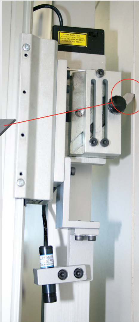
Blade cutting head powered by pneumatic linear actuator. Shown here with optional laser sighting system
