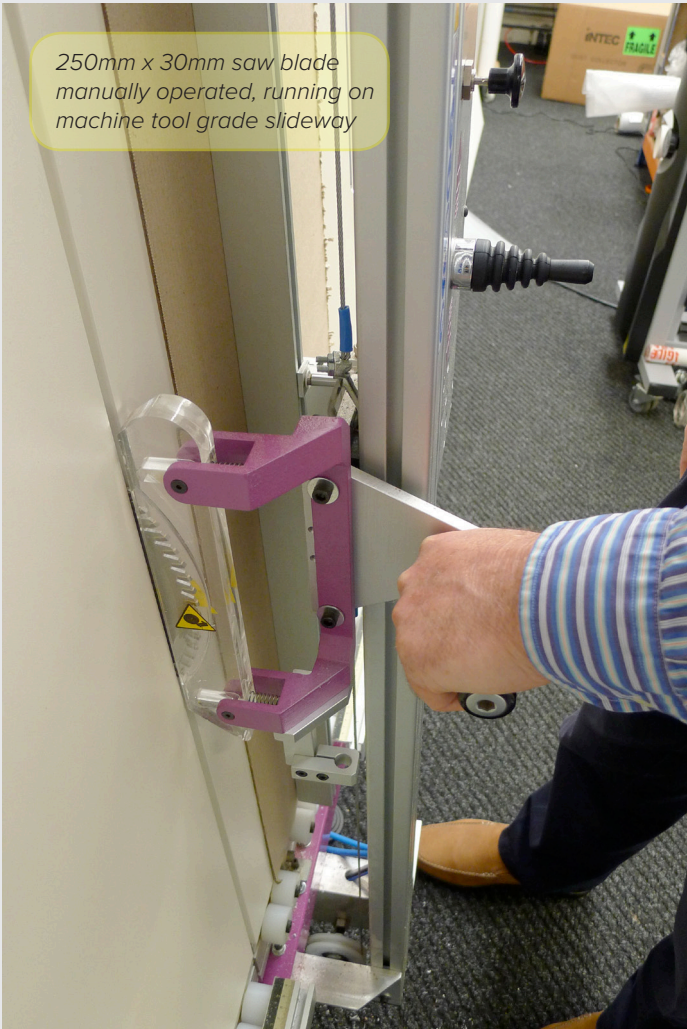
Blade cutting head powered by pneumatic linear actuator. Shown here with optional laser sighting system
